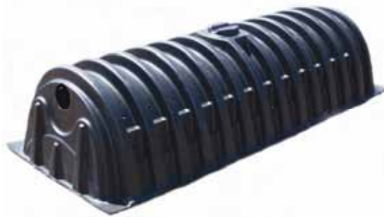
ecoChamber 2036 – Low Profile Chamber 36" wide X 20" tall and 5.7 cubic feet of water storage (per linear feet of lay length) when installed with 6" of stone base.
