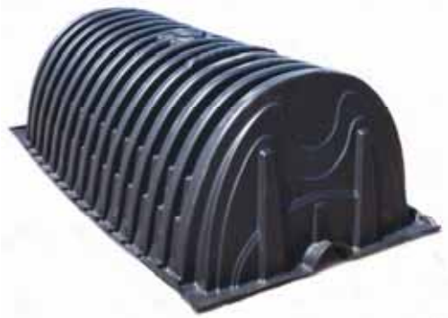
ecoChamber 3052 – High Capacity Chamber 52" wide X 30.5" tall and 11.3 cubic feet of water storage (per linear feet of lay length) when installed with 6" of stone base.
